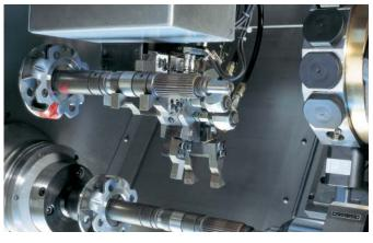
The workpiece handling for longer shaft parts
