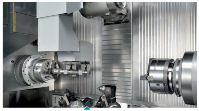
The integrated workpiece handling unit is available as an option. It can be used for loading and unloading as well as for the removal of remnants and is suitable for parts weighing up to 20 kg and with a diameter of up to D 120 mm.
